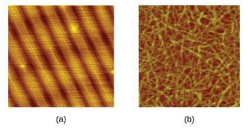
**Figure 1.28** STMs and AFMs allow us to view images at the atomic level. (a) This STM image of a pure gold surface shows individual atoms of gold arranged in columns. (b) This AFM image shows long, strand-like molecules of nanocellulose, a laboratory-created substance derived from plant fibers. (credit a: modification of work by "Erwinrossen"/Wikimedia Commons)
