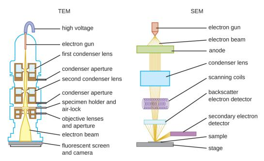
Figure 1.24 These schematic illustrations compare the components of transmission electron microscopes and scanning electron microscopes.
