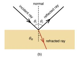
Figure 1.4 (a) Refraction occurs when light passes from one medium, such as air, to another, such as glass, changing the direction of the light rays. (b) As shown in this diagram, light rays passing from one medium to another may be either refracted or reflected. (credit a: modification of work by "ajizai"/Wikimedia Commons)
