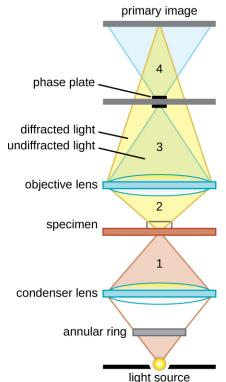
**Figure 1.17** This diagram of a phase-contrast microscope illustrates phase differences between light passing through the object and background. These differences are produced by passing the rays through different parts of a phase plate. The light rays are superimposed in the image plane, producing contrast due to their interference.
