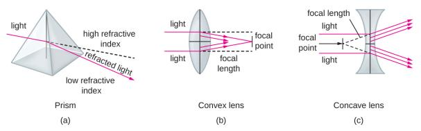
Figure 1.6 (a) A lens is like a collection of prisms, such as the one shown here. (b) When light passes through a convex lens, it is refracted toward a focal point on the other side of the lens. The focal length is the distance to the focal point. (c) Light passing through a concave lens is refracted away from a focal point in front of the lens.
