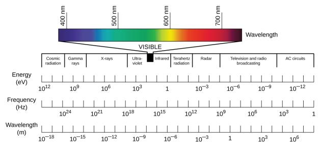
Figure 1.7 The electromagnetic spectrum ranges from high-frequency gamma rays to low-frequency radio waves. Visible light is the relatively small range of electromagnetic frequencies that can be sensed by the human eye. On the electromagnetic spectrum, visible light falls between ultraviolet and infrared light. (credit: modification of work by Johannes Ahlmann)
