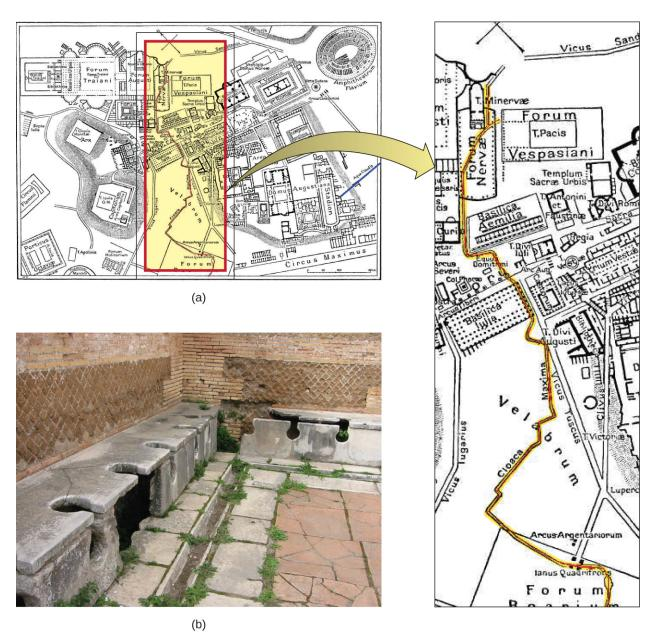
**Figure 1.4** (a) The *Cloaca Maxima*, or "Greatest Sewer" (shown in red), ran through ancient Rome. It was an engineering marvel that carried waste away from the city and into the river Tiber. (b) These ancient latrines emptied into the *Cloaca Maxima*.
