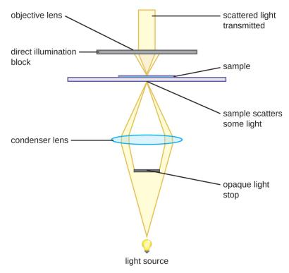
**Figure 1.15** An opaque light stop inserted into a brightfield microscope is used to produce a darkfield image. The light stop blocks light traveling directly from the illuminator to the objective lens, allowing only light reflected or refracted off the specimen to reach the eye.
