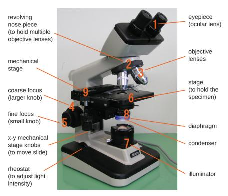
Figure 1.13 Components of a typical brightfield microscope.
